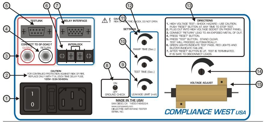
Figure 2. Rear Panel Controls, Indicators and Connectors
