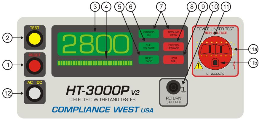
Figure 1. Front Panel Controls, Indicators and Connectors for HT-2000P V2, HT-2800P V2 and HT-3000P V2.
