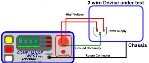
Figure 7. Testing a Three Wire Power Cord Device.
