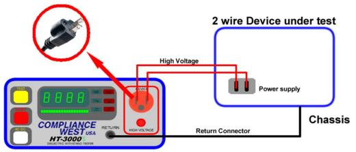
Figure 8. Testing a Two Wire Power Cord Device
