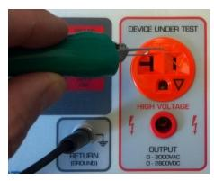
5. The test should immediately terminate with a buzzer. The Ground OK, Ground Open, Full Voltage, Hipot Fail and red RESET LED's should be lit.
